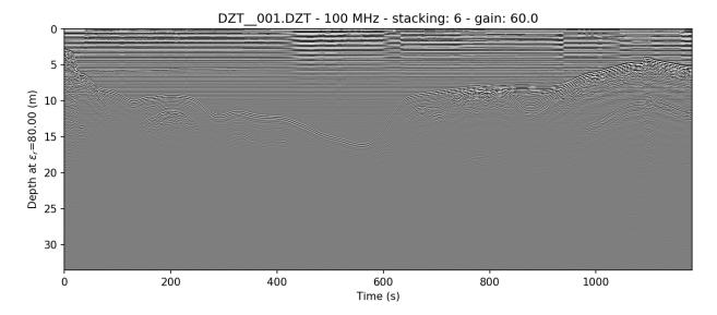
If you would like to learn how to remove the horizontal noise in the water column of this image, head to *Getting rid of horizontal noise*.
